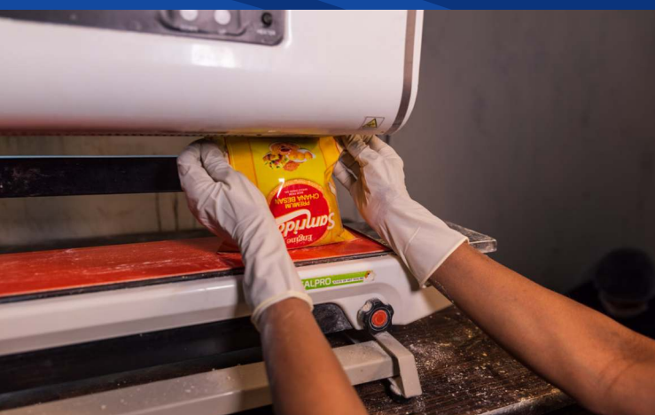
Manual packing section for Maida / Suji / Dalia / Besan in pre-formed pouches
