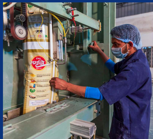
2 Nos. VFFS machines for packing 10kg/ 5kg/1kg atta with pouch pressing conveyors
